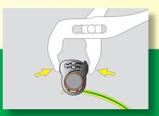
The two first teeth of the jaw have been designed to allow the clamp to be tightened initially by hand, and once clamp is positioned in desired location the fastening operation is completed by pliers. Locking tabs prevent release of the jaws once the clamp is secured.
