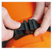
STEP 2: Wrap band around application and pull through free end of buckle. Pull band tight by hand
