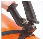
STEP 4: Trim off excess band using cutting blade
