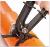
STEP 3: Squeeze handles together to tighten band
