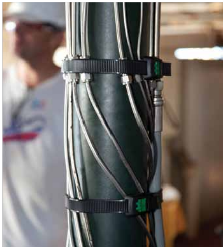
Photo courtesy of William Crawford and IODP-USIO Smart Ties holding the maze of tubing lines feeding into downhole packers
